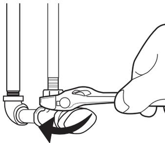
**2** Disconnect the cold water hose from the line. Make sure it is the cold water hose and not hot because hot water will cause the unit to malfunction.
