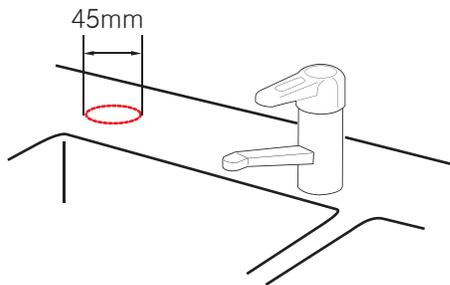
**1** Use appropriate tools to make 45mm diameter hole in the location where you will set up the faucet. Make sure the faucet location will allow both spouts to reach the sink.
