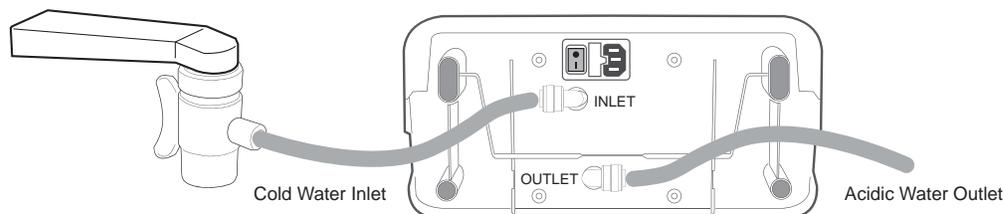
**5** Connect hoses to the water Inlet and Acidic water Outlet.
