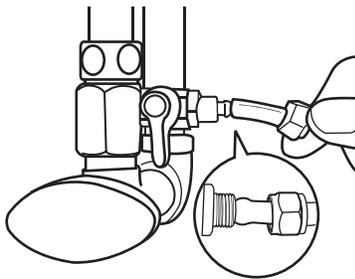
**5** Connect the plastic tubing as shown.
