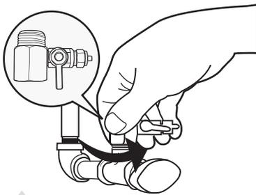
**4** Connect the cold water line adapter to the cold water supply valve as shown. As fittings vary you will need to find the right size adapters at your local plumbing store.
