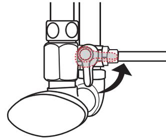
**6** Connect hoses to the water inlet and acidic water outlet then open the cold water supply valve.
