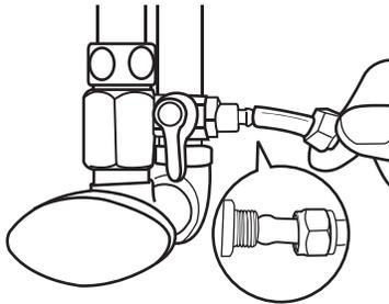
**5** Connect the plastic tubing as shown.
