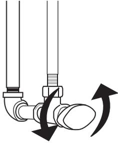
**1** Find the cold water supply line and close the valve.
