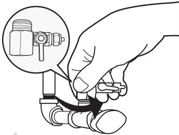
**4** Connect the cold water line adapter to the cold water supply valve as shown. As fittings vary you will need to find the right size adapters at your local plumbing store.
